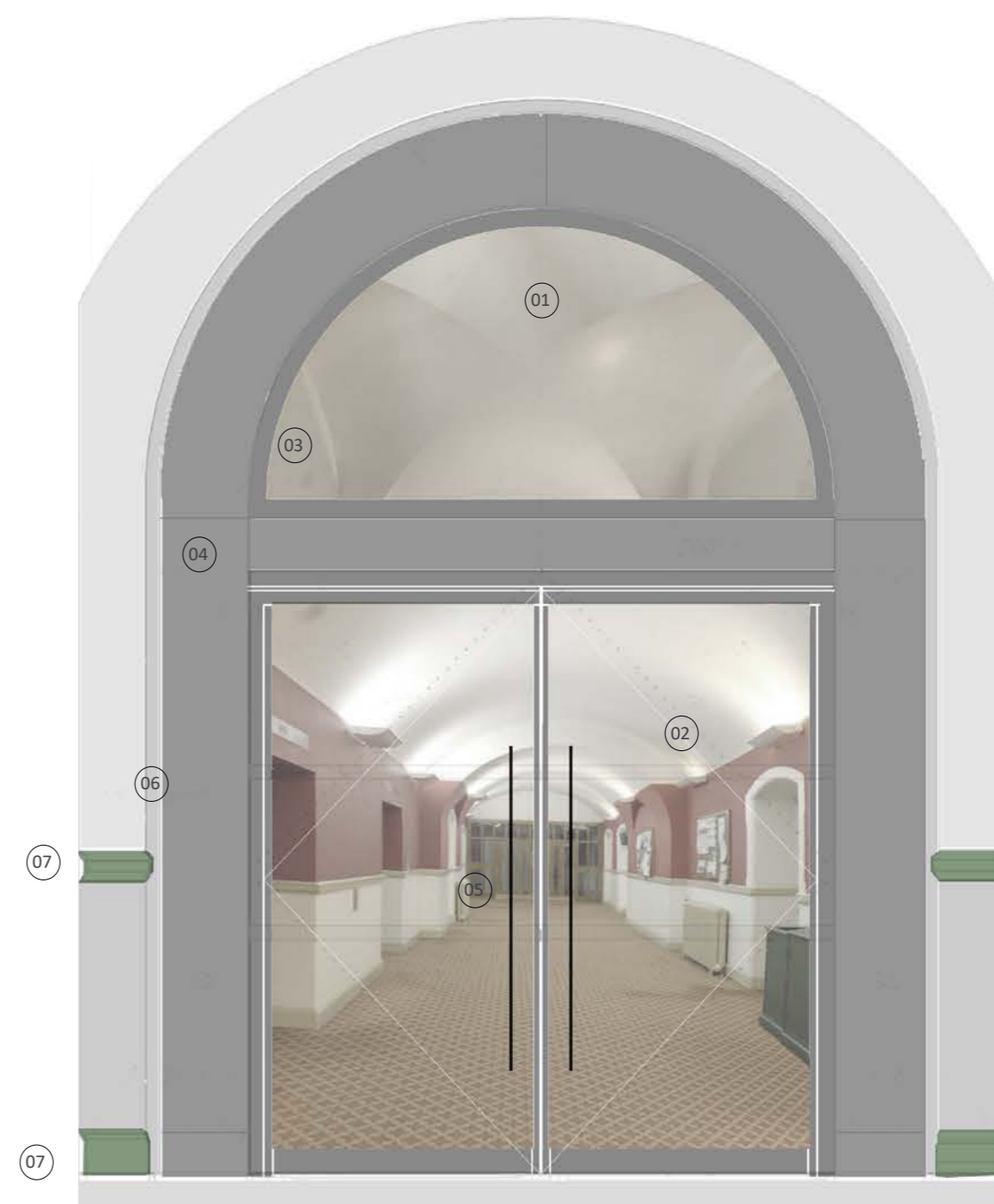
Design intent for glazed fire doors and screens typically to be used in areas of highest heritage significance
