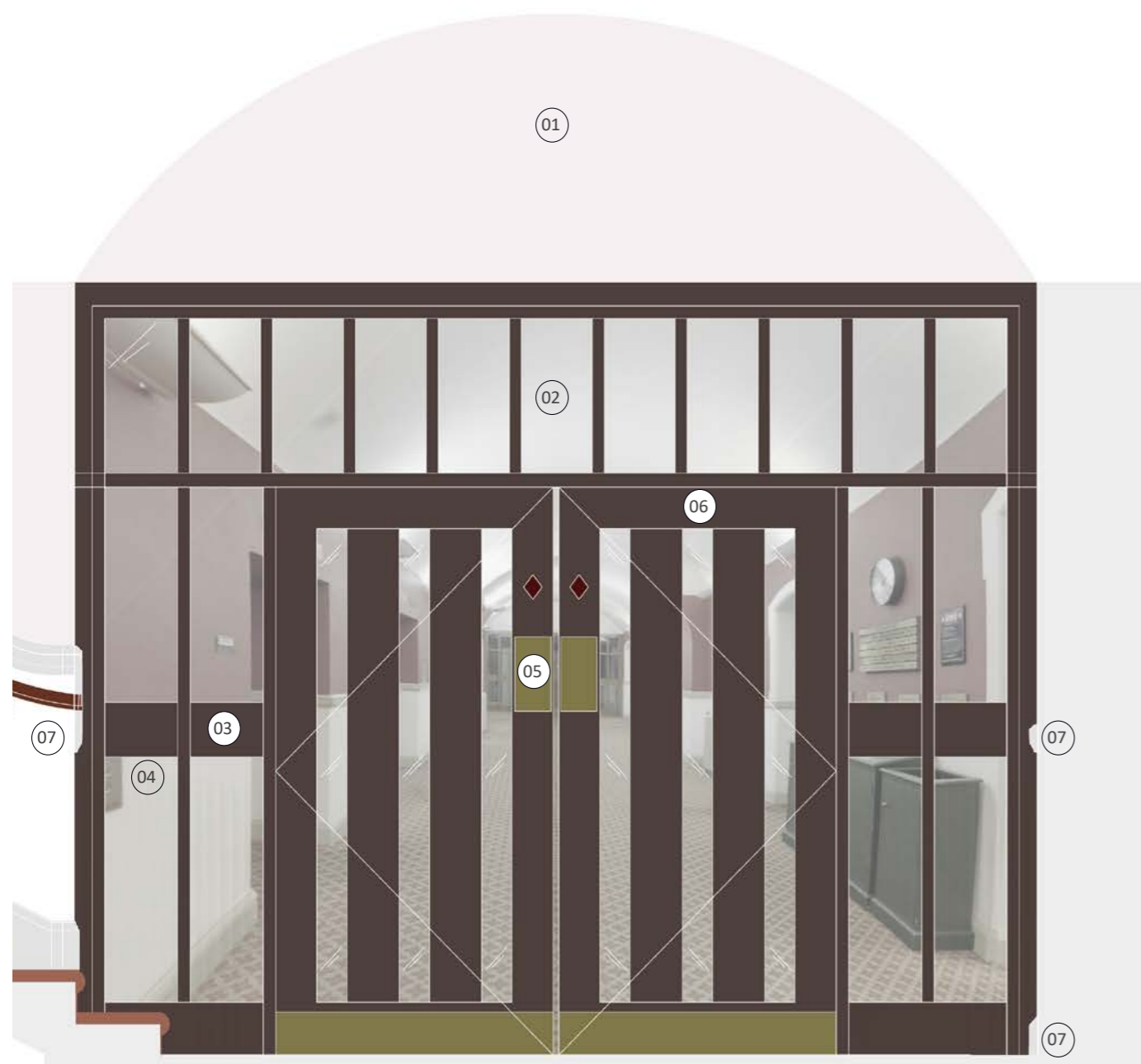
Existing 1970s timber glazed doors and glazed overhead
