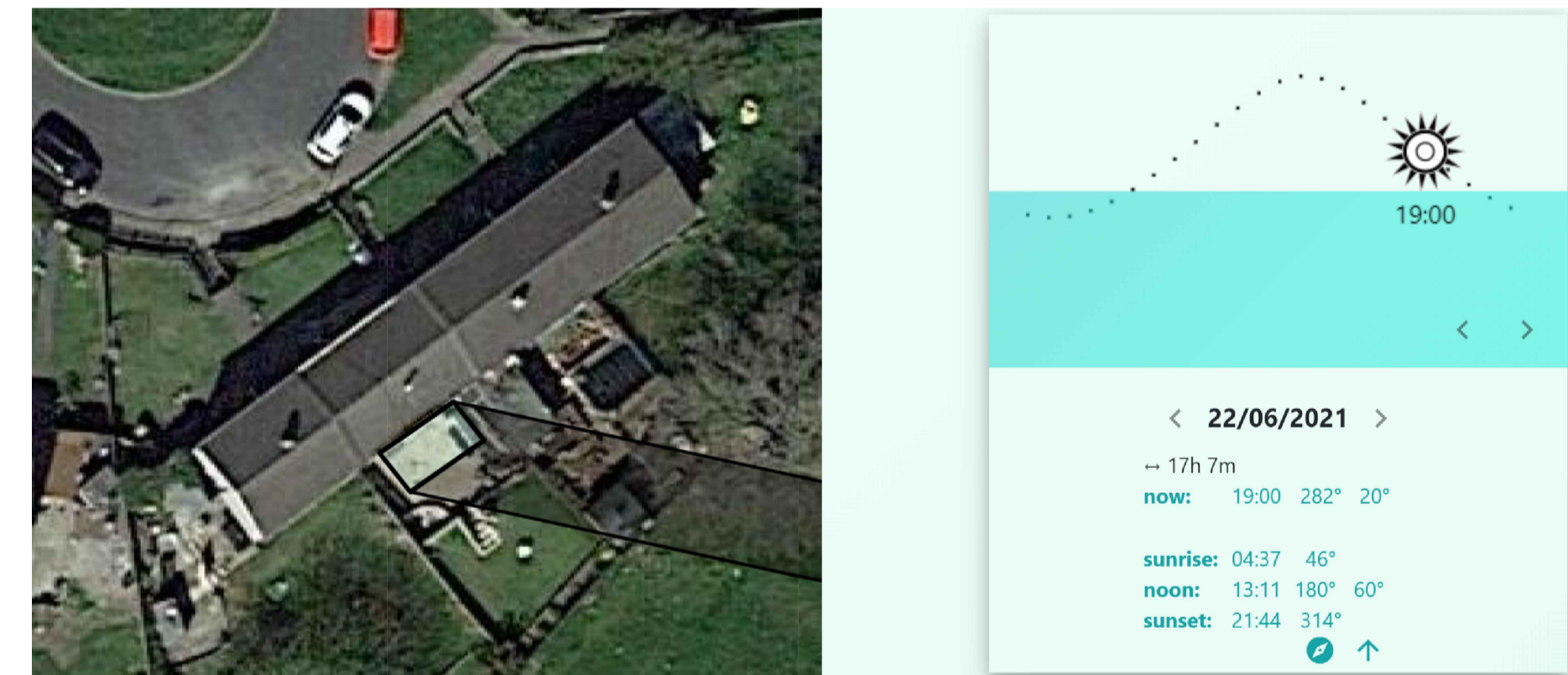
SHADOW FROM PROPOSED EXTENSION 19:00 22/06/2021, MID SUMMER NOTE-SHADOW FROM EXISTING HOUSE NOT DETAILED
