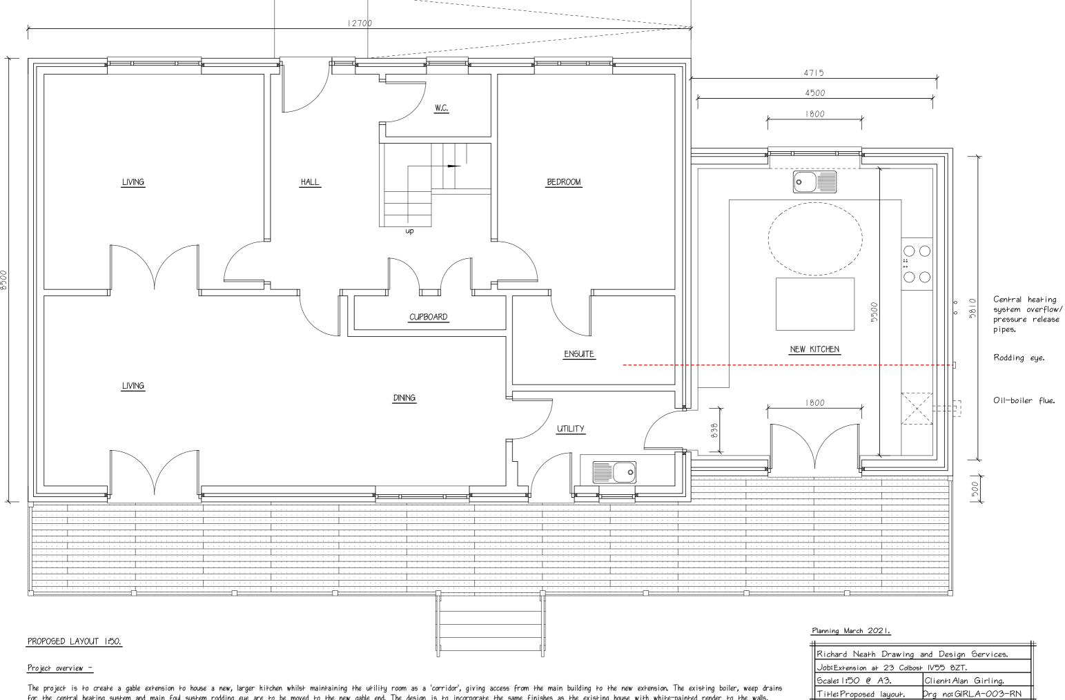
for the central heating system and main foul system rodding eye are to be moved to the new gable end. The design is to incorporate the same finishes as the existing house with white-painted render to the walls, white PVCu windows, concrete interlocking roof tiles and black rainwater goods. Decking is to be composite boarding and handrails/balusters, with timber posts. All services are on site and existing accessible facilities are in order.
