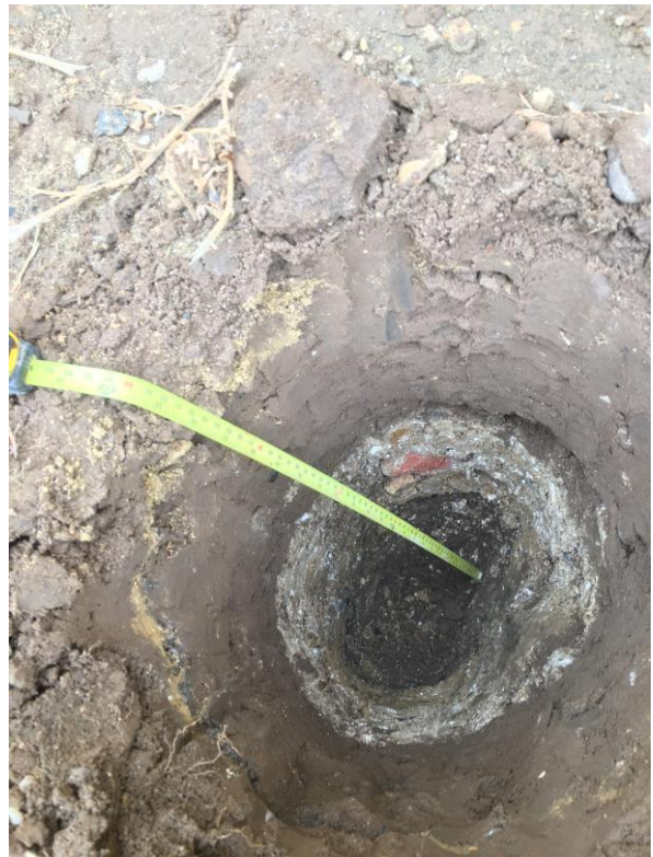
Photographs 1 - 4 , taken on the 27 th July 2020 showing the depth and nature of the subsoil and topsoil within the cover systems for plots 240 to 243 and flats 244 to 249.
