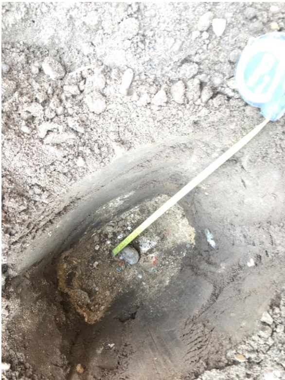
Photographs 1 - 4 , taken on the 27 th July 2020 showing the depth and nature of the subsoil and topsoil within the cover systems for plots 240 to 243 and flats 244 to 249.
