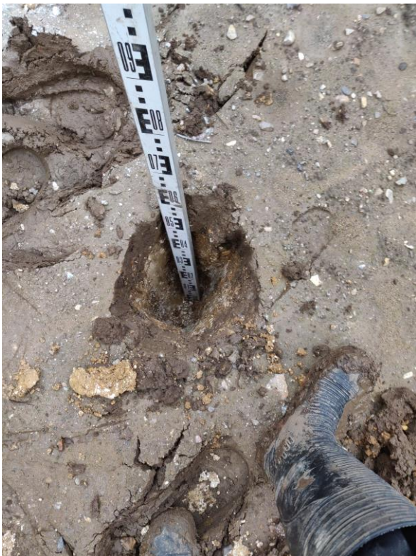
Photographs 10 and 11 , taken on the 10 th December 2019, showing the depth and nature of subsoil and topsoil within the garden areas of plots 265 and 266 (HDT265-03 and HDT266-02).
