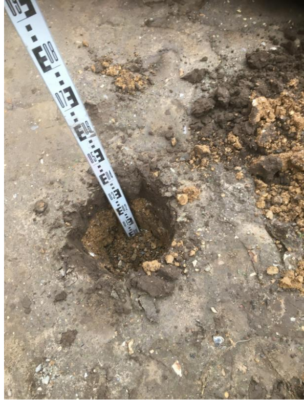
Photographs 8 and 9 , taken on the 10 th December 2019 showing where pea shingle and coarse gravel were encountered within hand dug trial pits (HDT262-03 and HDT266-01) and presumed to indicate the presence of services.
