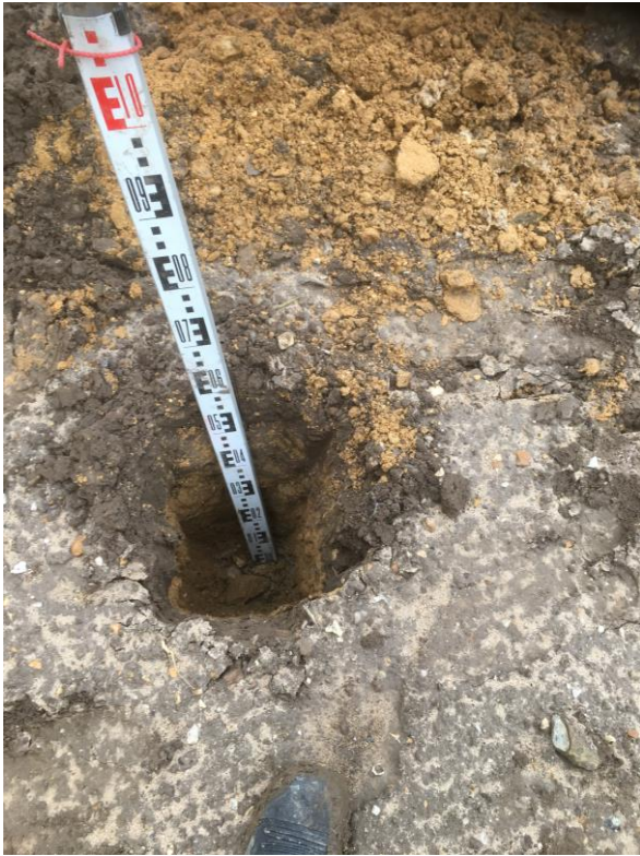
Photographs 1 - 2 , taken on the 10 th December 2019, showing the depth and nature of subsoil and topsoil within the rear garden area of plot 256 (HDTP256-02 and HDTP256-04).
