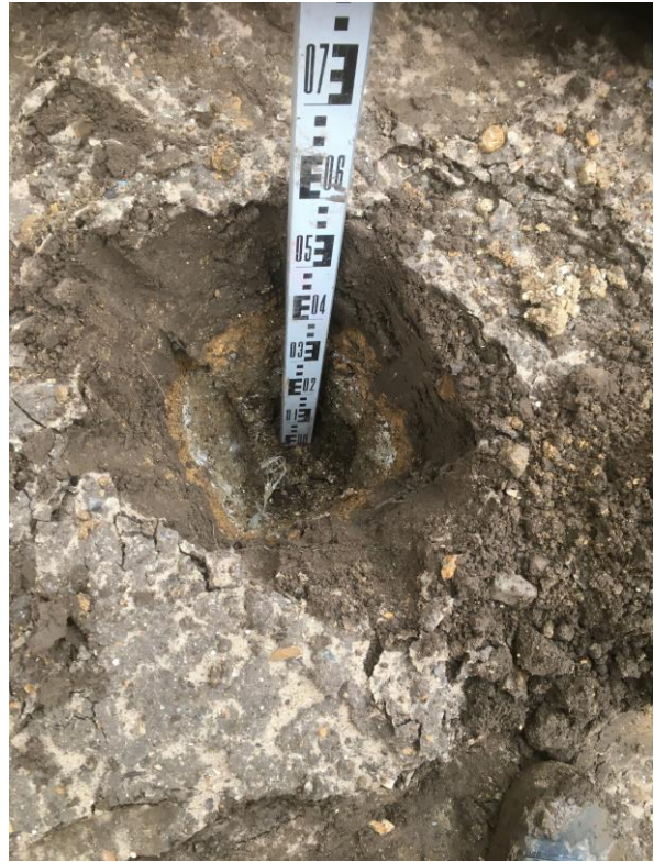
Photographs 1 - 2 , taken on the 10 th December 2019, showing the depth and nature of subsoil and topsoil within the rear garden area of plot 256 (HDTP256-02 and HDTP256-04).
