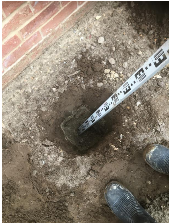
Photographs 6 and 7 , taken on the 3 rd and 10 th December 2019, showing the depth and nature of subsoil and topsoil within the garden areas of plots 260, 261 and 262 (HOTP260-01 and HOTP261-03).
