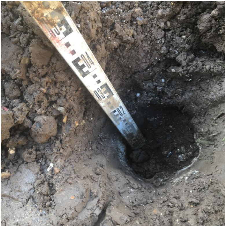
Photograph 9 , taken on the 3 rd December 2019, showing the depth and nature of the darker subsoil encountered in plot 258 (HDTP258-05) that was proven to be chemically suitable to remain as part of the cover system.
