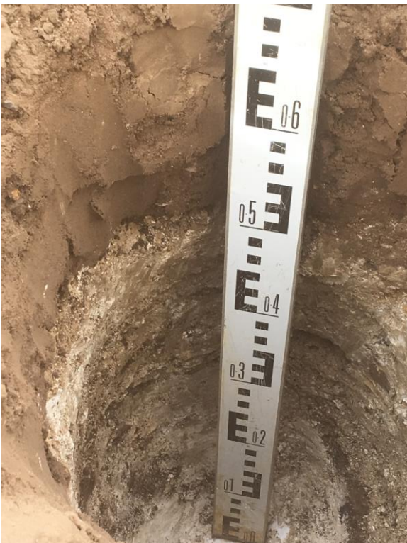
Photographs 1 - 4 , taken on the 2 nd September 2019, showing the depth and nature of subsoil and topsoil within the back garden of plot 169 (HOTP169-03) and the arisings generated.
