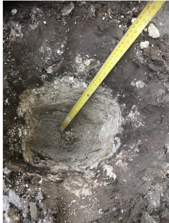
Photographs 1 - 2 , taken on the 4 th February 2020, showing the depth and nature of subsoil and topsoil within the front and rear garden area of plot 250 (HDTP250-06 and HDTP250-04).
