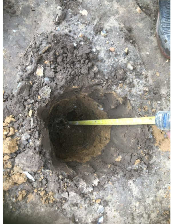
Photographs 9 - 10 , taken on the 4 th February 2020, showing the depth and nature of subsoil and topsoil within the front and rear garden areas of plots 264 (HDTP264-01 and HDTP264-05).
