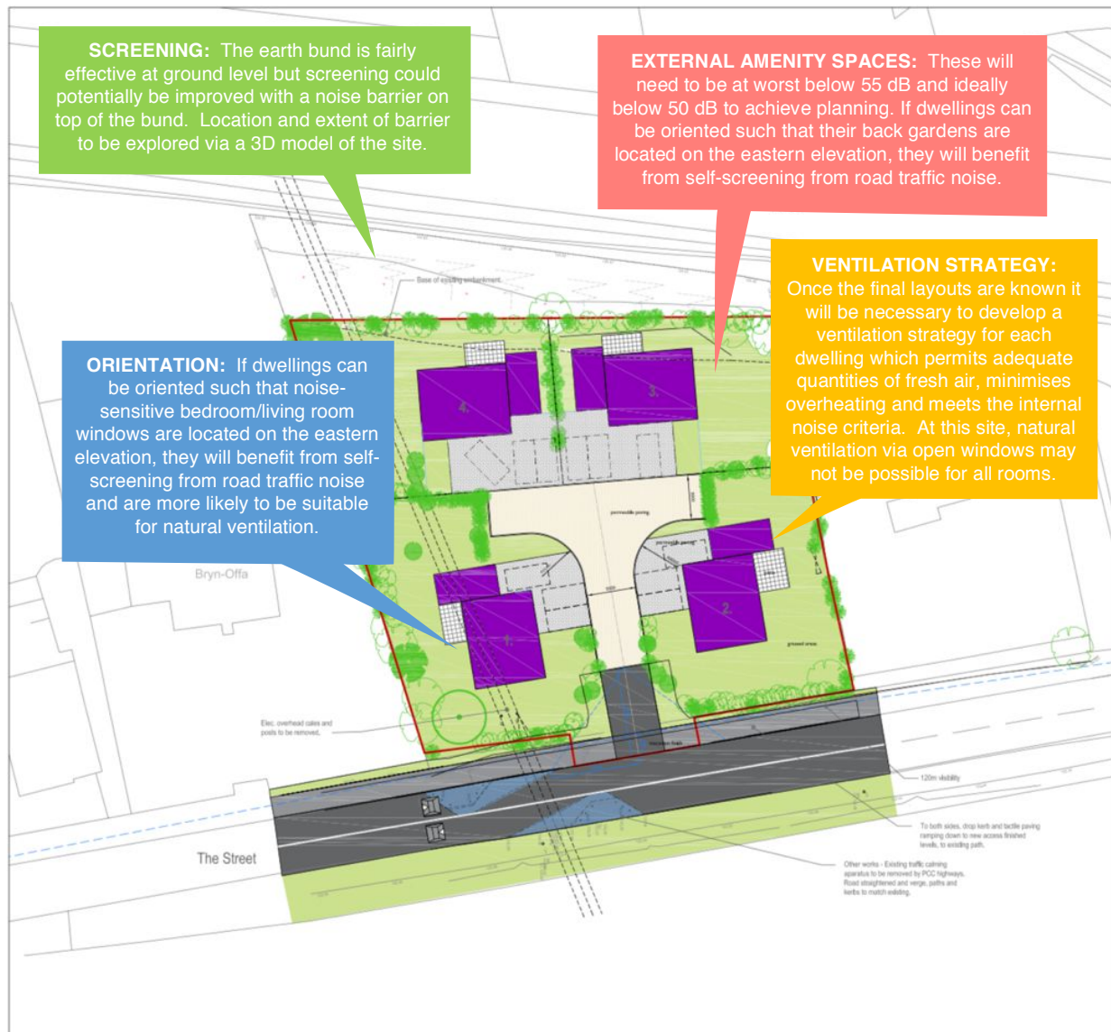
Figure 5 Indicative site layout and good acoustic design measures to be addressed during the next stage.
