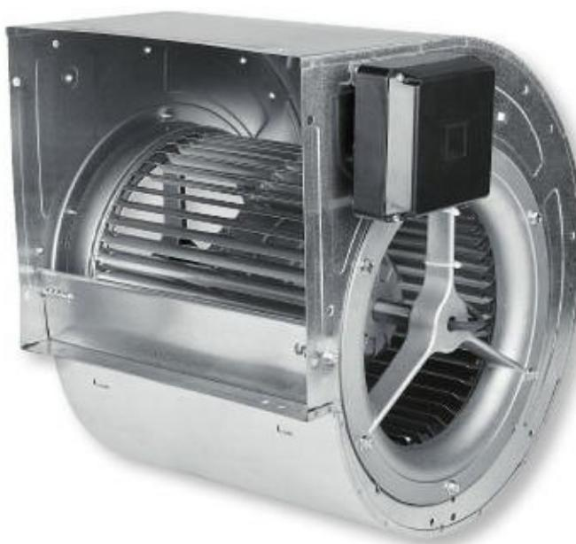
Range of direct-driven low pressure double inlet forward curve centrifugal fans. Casing and impeller manufactured from galvanized sheet steel.
