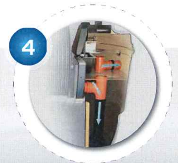
FINAL SETTLEMENT TANK The clean liquid passes into the final settlement tank where it can be discharged to ground or water course.
