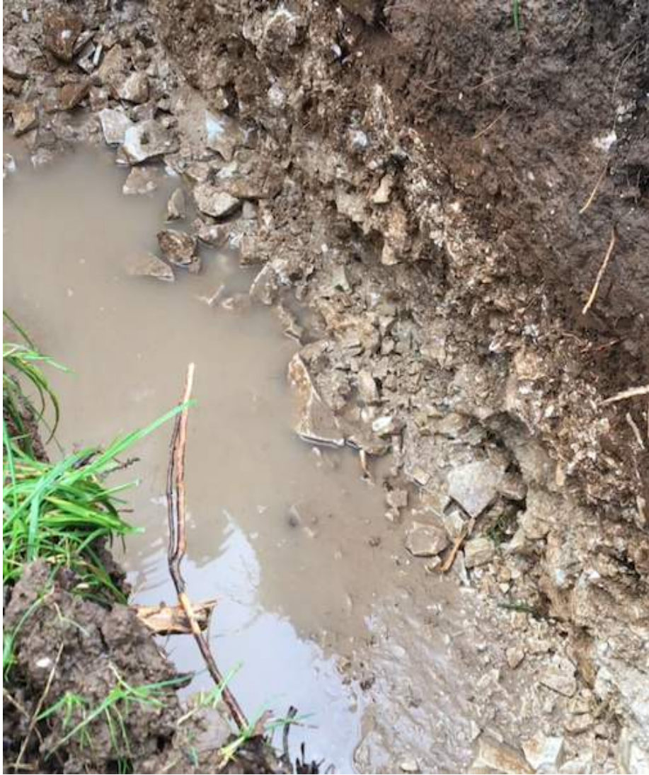
The above photo shows the test hole depth immediately following the completion of discharge of 1.1 cubic meters of water.
