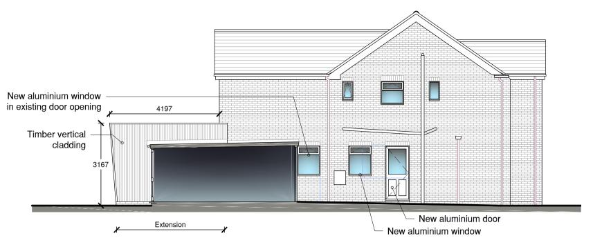
Sectional Side (South) Elevation Scale 1:100
