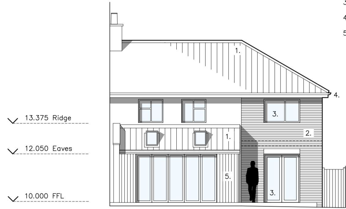
Proposed Rear Elevation Scale 1:100
