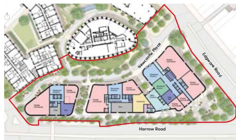
Proposed ground floor plan, showing new landscaped Newcastle Place and range of ground floor uses.
