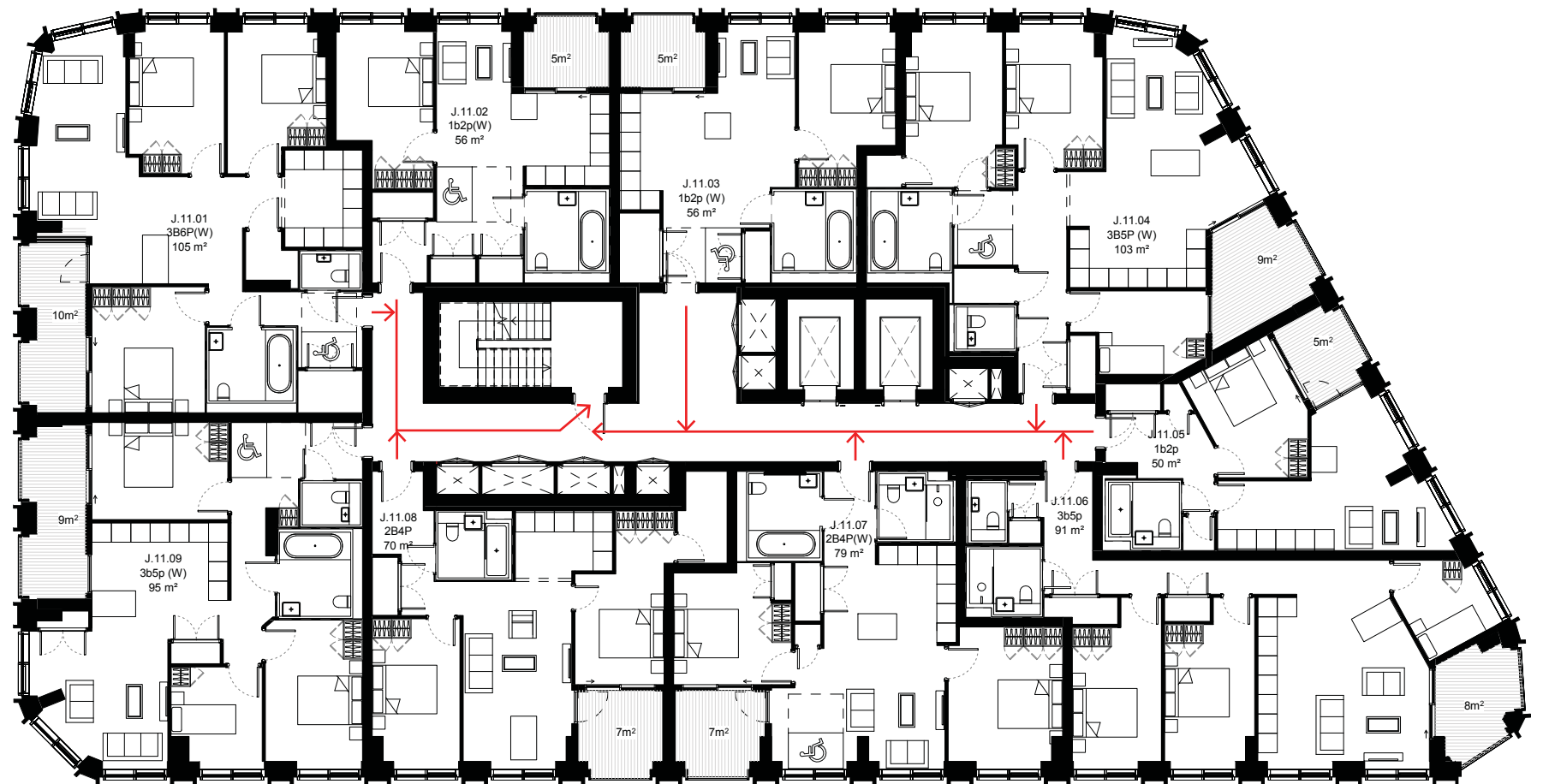
Fig. 5.50 Block J - Typical Floor - Fire Escape Routes
