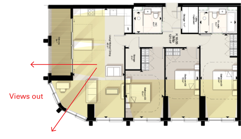
Fig. 5.29 Internal daylight/sunlight - Typical 3 bed / 6 person apartment
