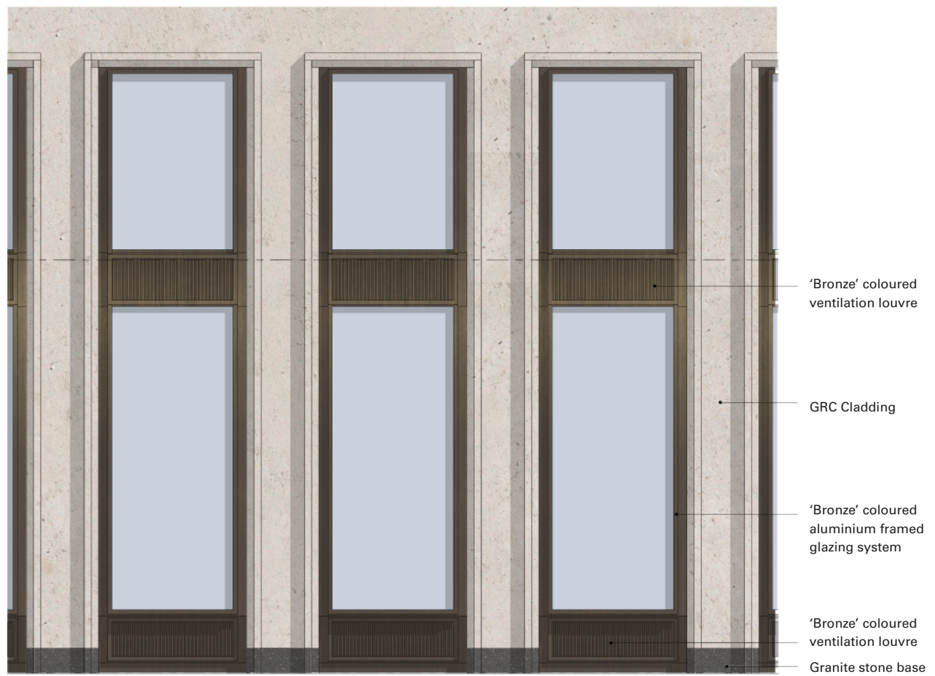
Fig. 5.16 Block K Bay Study Elevations
