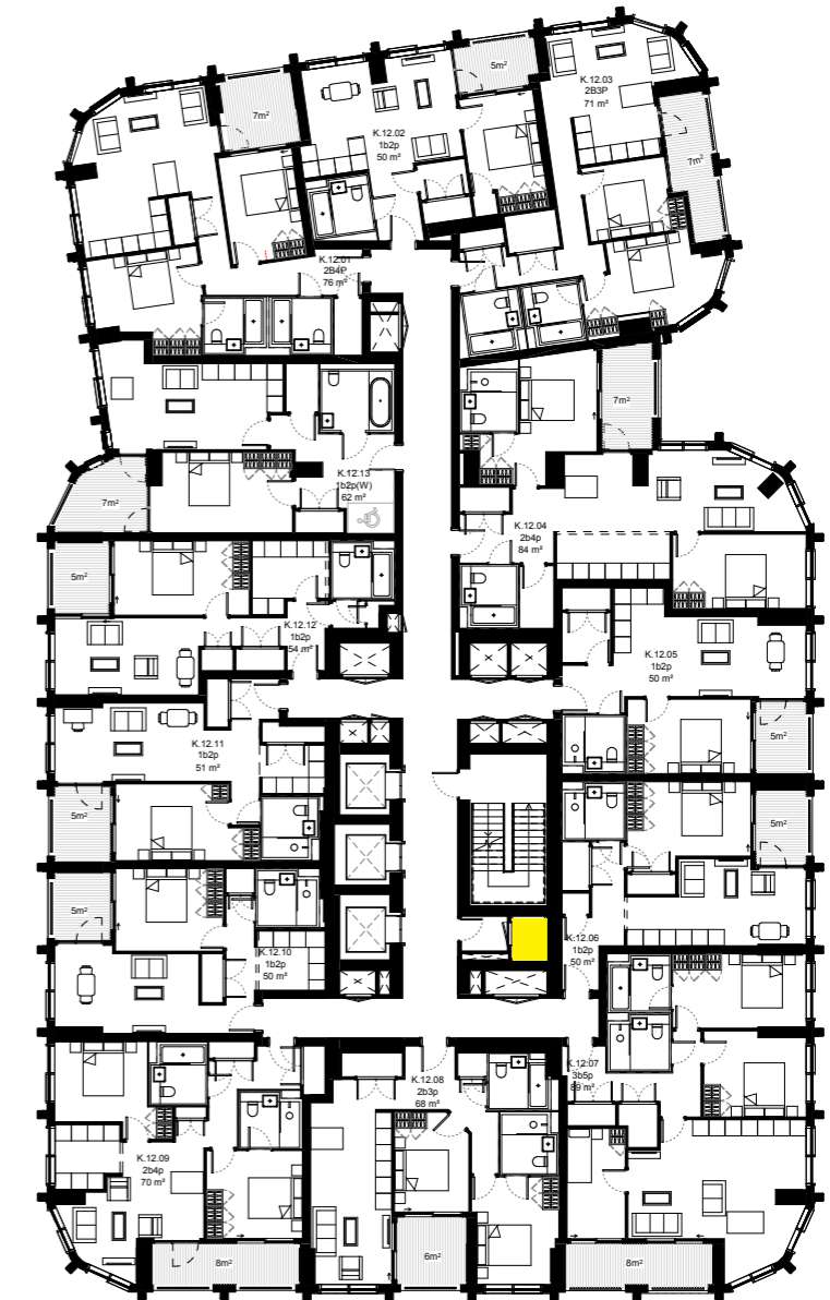
Figure 3.8 - Location of Waste Chute in Block K
