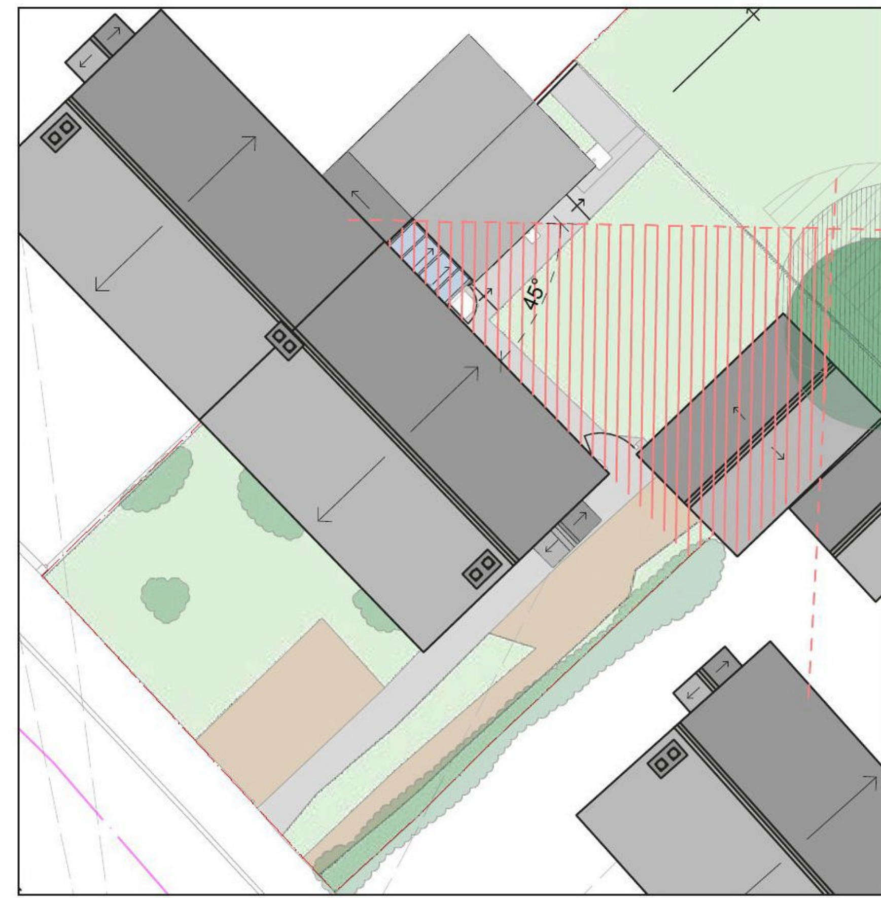
[Figure 48] Right to Light plan diagram showing potential area for development using 45degree rule from centre of adjacent window sills (Ref: OCC Sites and Housing Plan)
