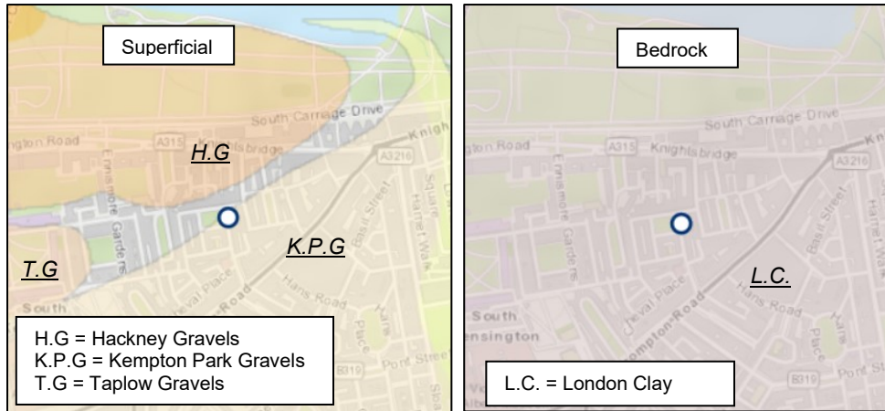
Figures 2 & 2a. Superficial and Bedrock geology of the Site (Ref. BGS Geoindex)
