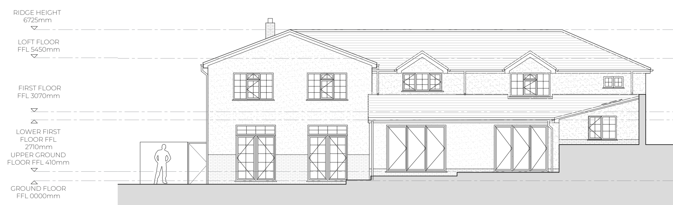
PROPOSED REAR (SOUTH) ELEVATION 1:100 @ A1
