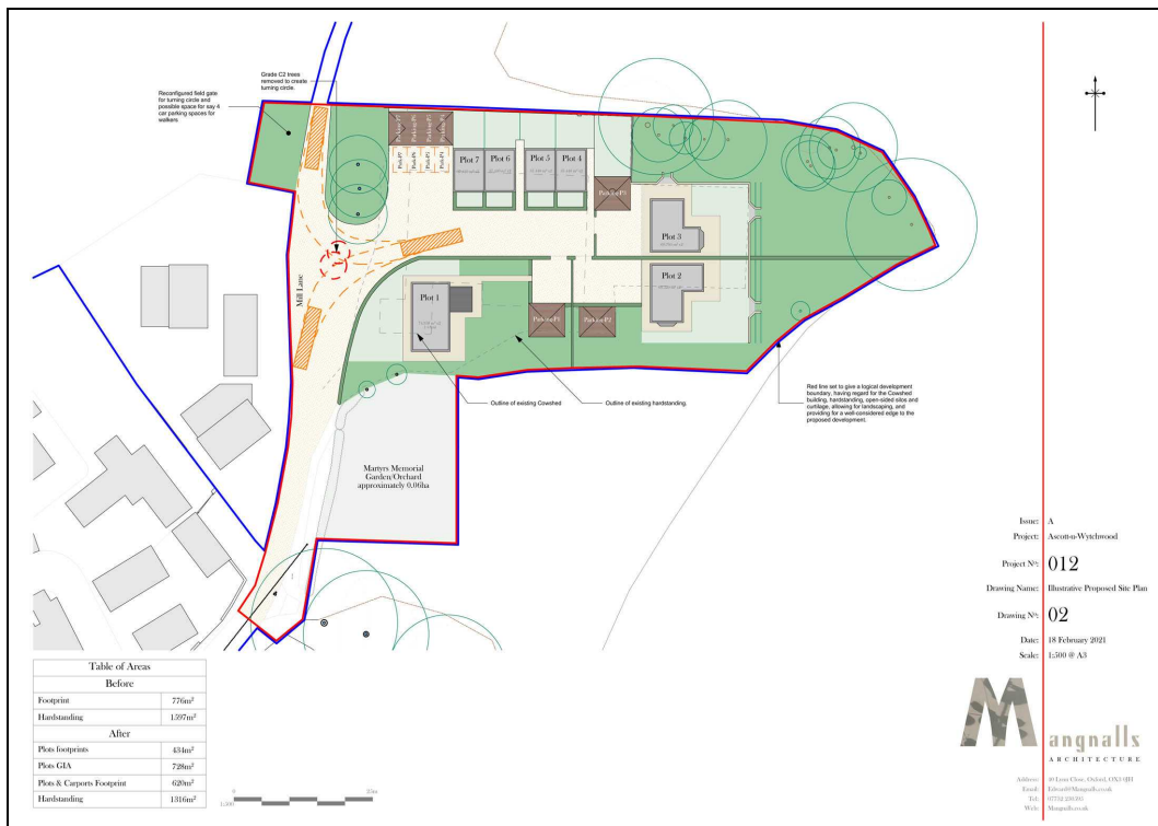
Figure 9 : Proposed Site Plan for re-development of the cow shed and yard at Yew Tree Farm.
