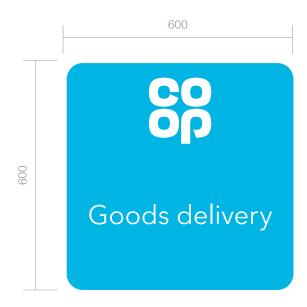
1No 3mm ACM with applied vinyl and anti-graffiti laminate. **Size:** 600x600mm
