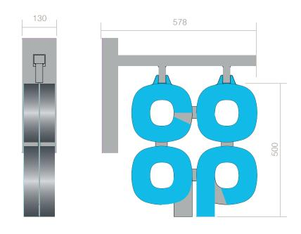
Internally Illuminated built up letters on both sides. Individual 3D letters constructed from silver aluminium side returns and Co-op BLUE acrylic faces - Internally illuminated by white LEDs (300 candelas) faces only to illuminate.
