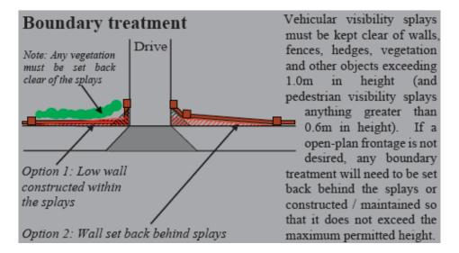
There should be no obstruction to visibility between heights of 0.85m and 2.0m above footway level. If the footway is likely to be used by small children, the height should be reduced to 0.6m. Where all or part of the splay lies across land outside of the applicant's control, a relaxation to this requirement may be considered, taking into account the amount of pedestrian activity along the footway and the width of the footway.
