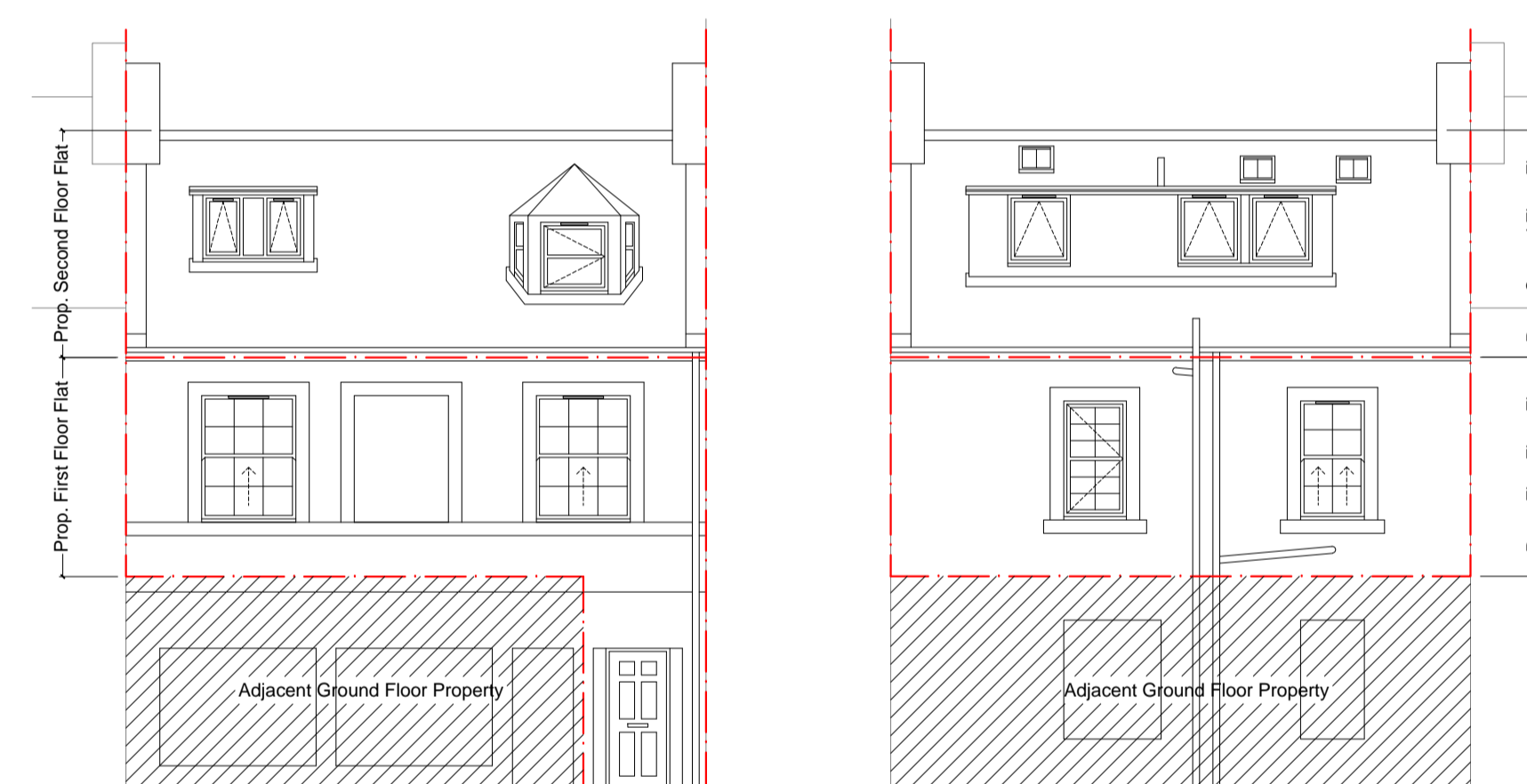
North - Front Elevation No physical changes proposed to elevation Proposed Elevations 1:100 at A1 1:100 (m) 0 1 5 10
