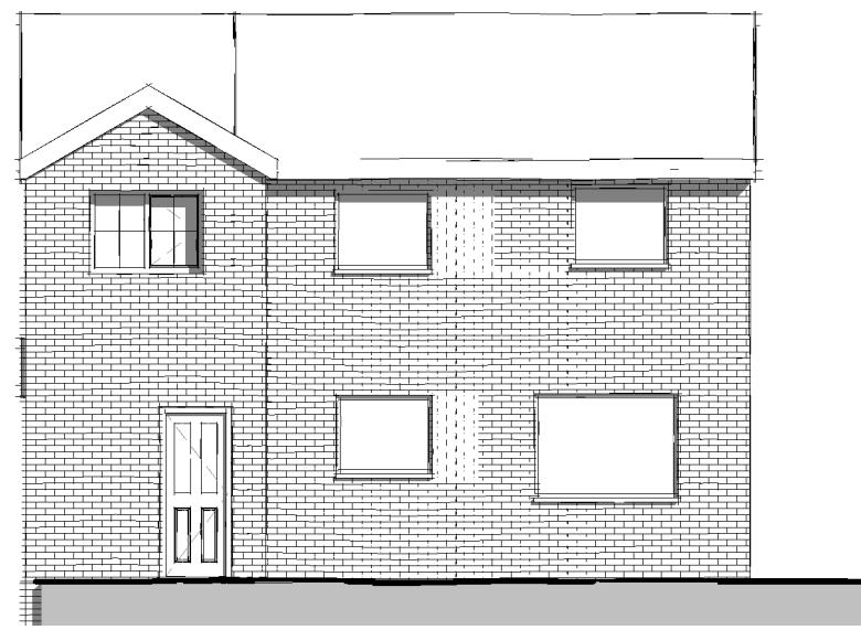
4 Proposed Rear Elevation 1 : 100
