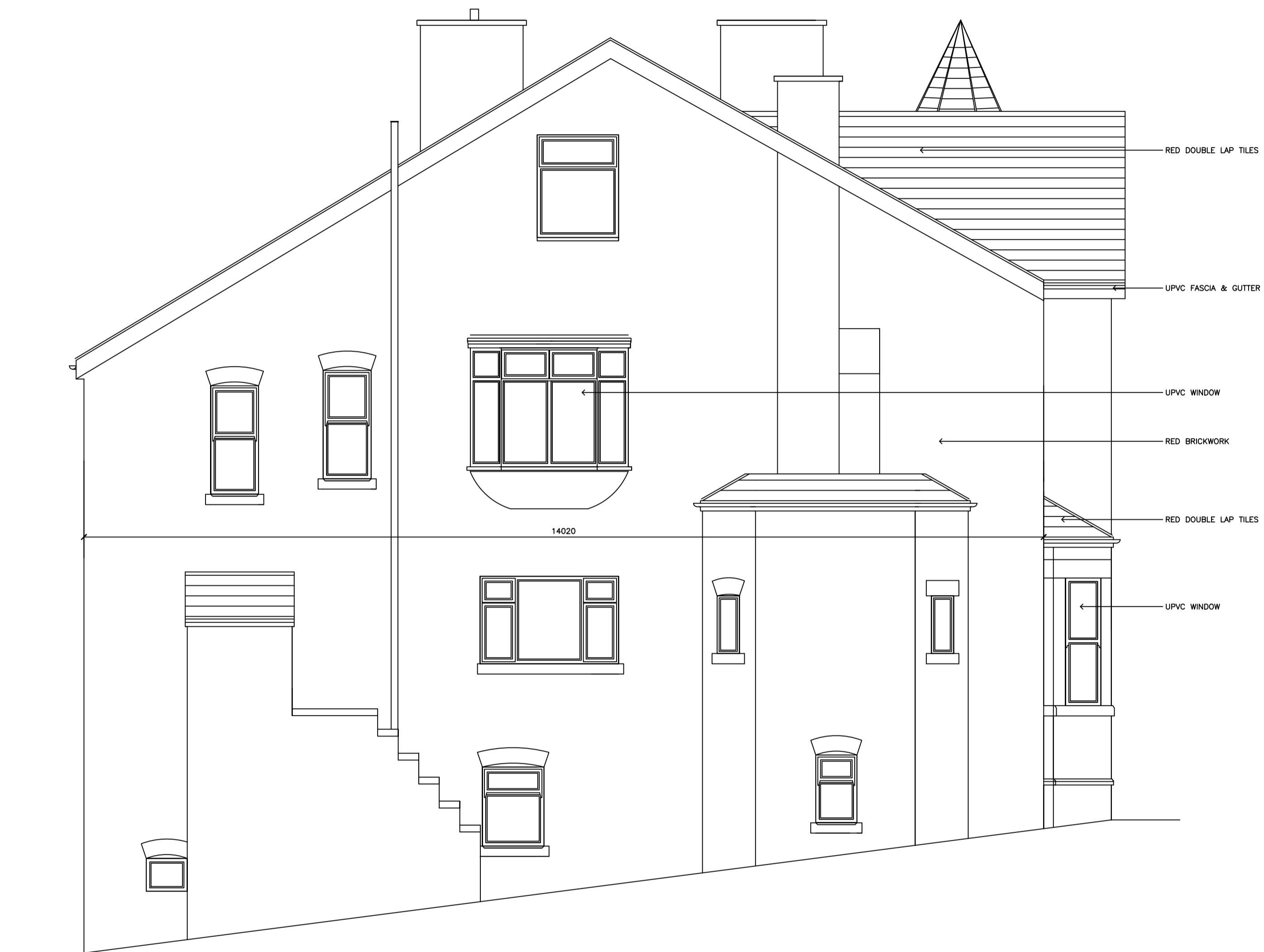
EXISTING BUILDING SIDE ELEVATION (SCALE 1:50)
