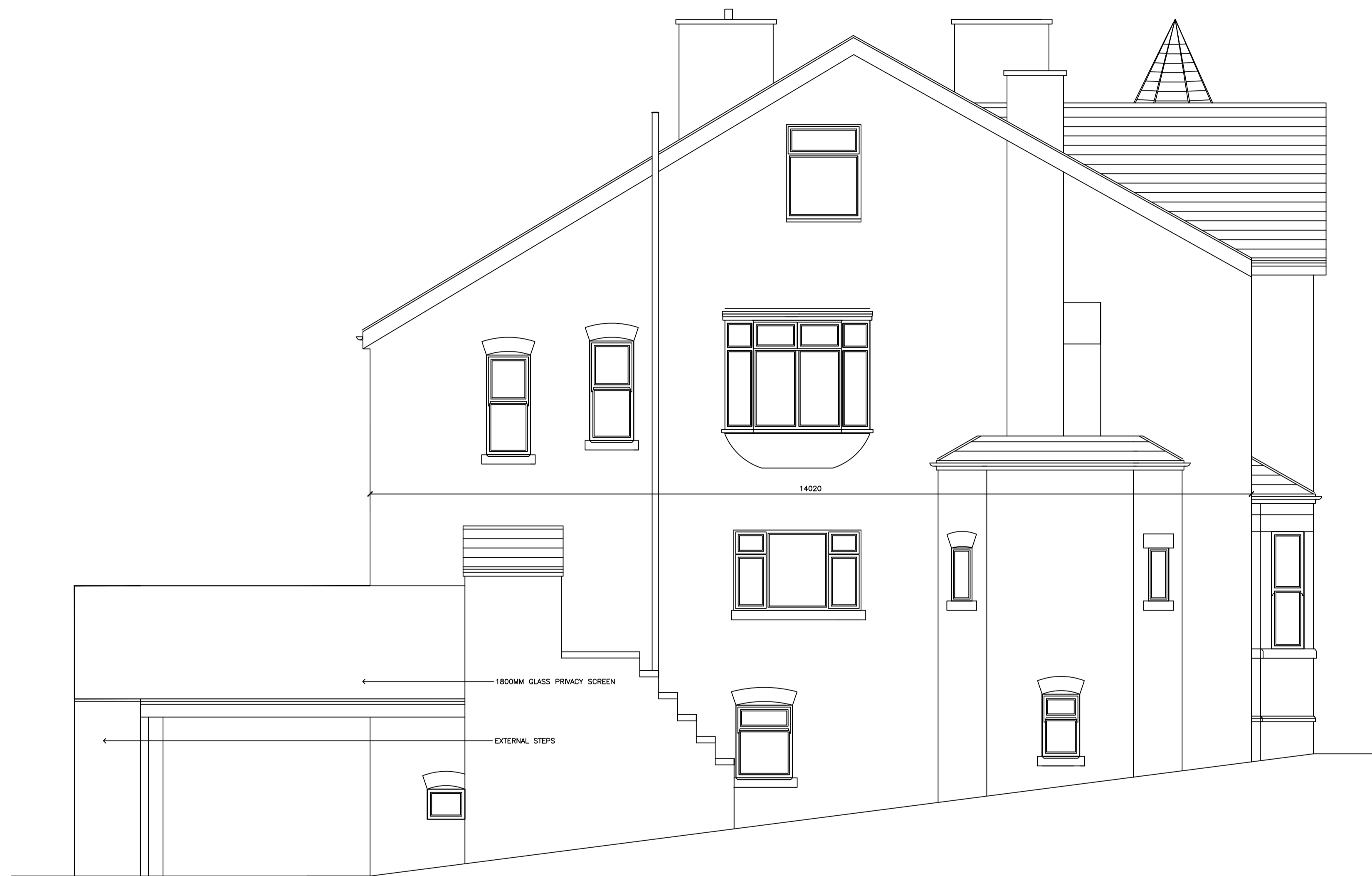
PROPOSED BUILDING SIDE ELEVATION (SCALE 1:50)
