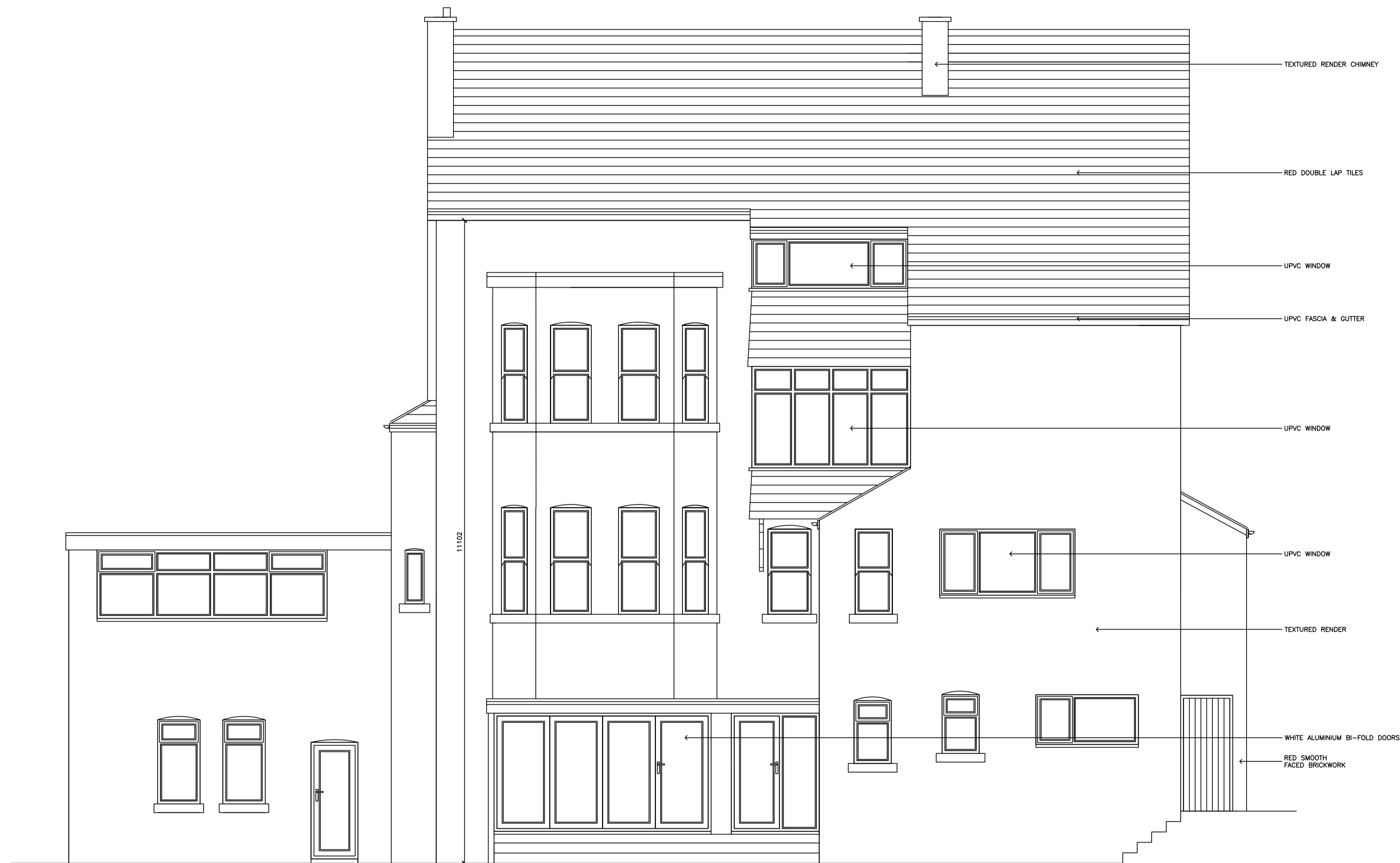
EXISTING BUILDING REAR ELEVATION (SCALE 1:50)
