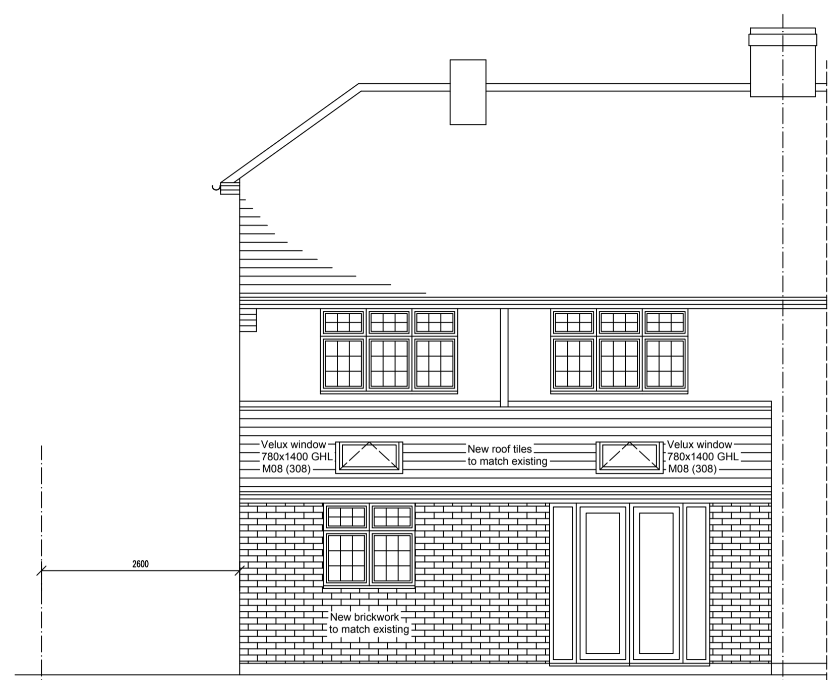
PROPOSED REAR ELEVATION (scale 1:50)
