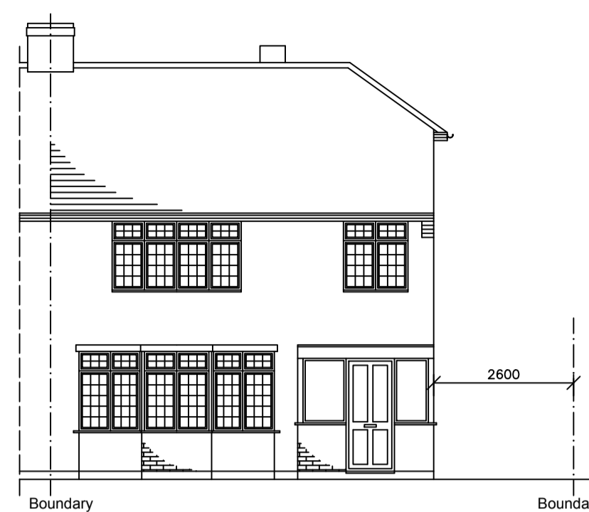
EXISTING FRONT ELEVATION (scale 1:100)
