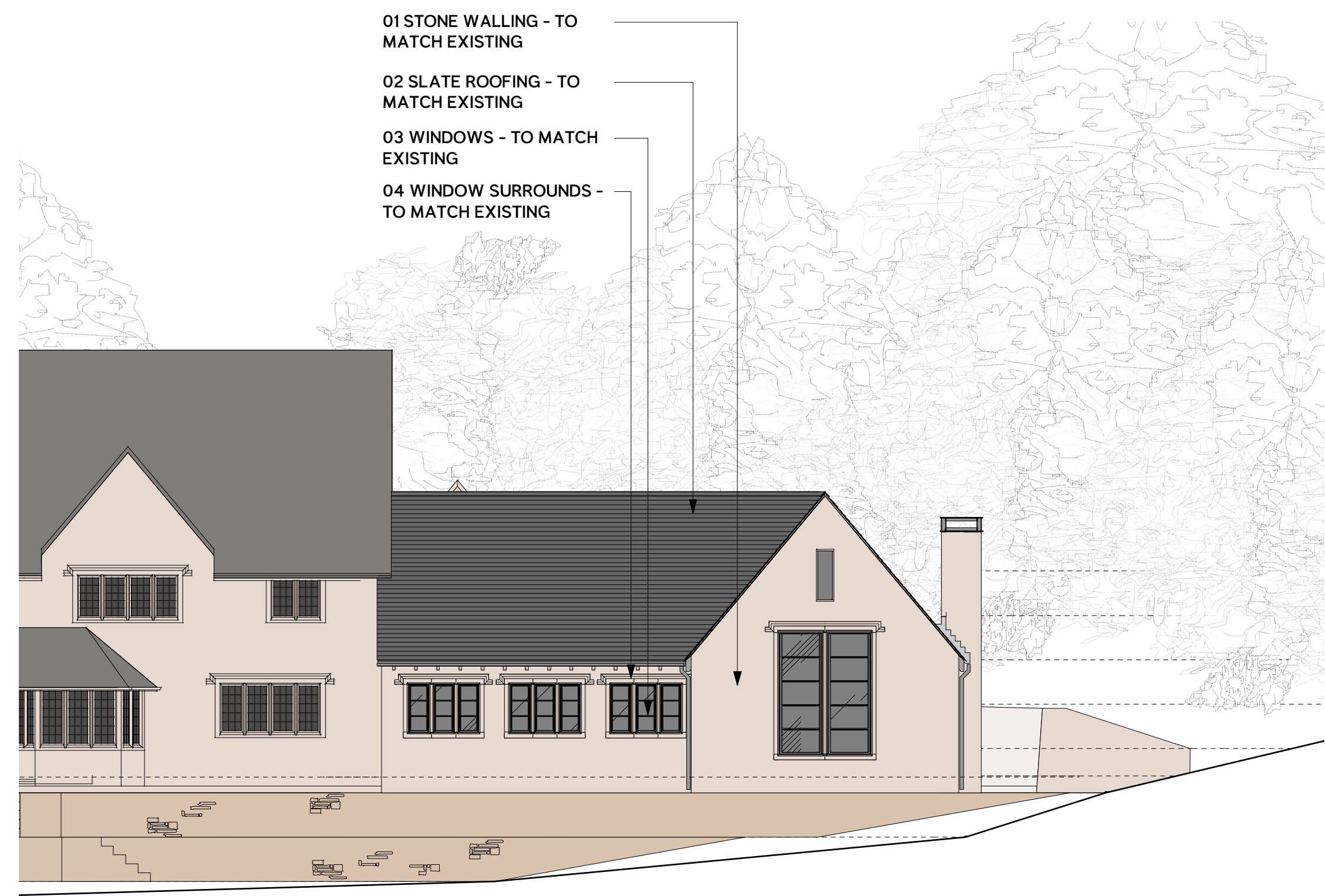
01 PROPOSED SOUTH FACING PARTIAL ELEVATION SHOWING NEW EXTENSION 1:100 @ A1 / 1:200 @ A3
