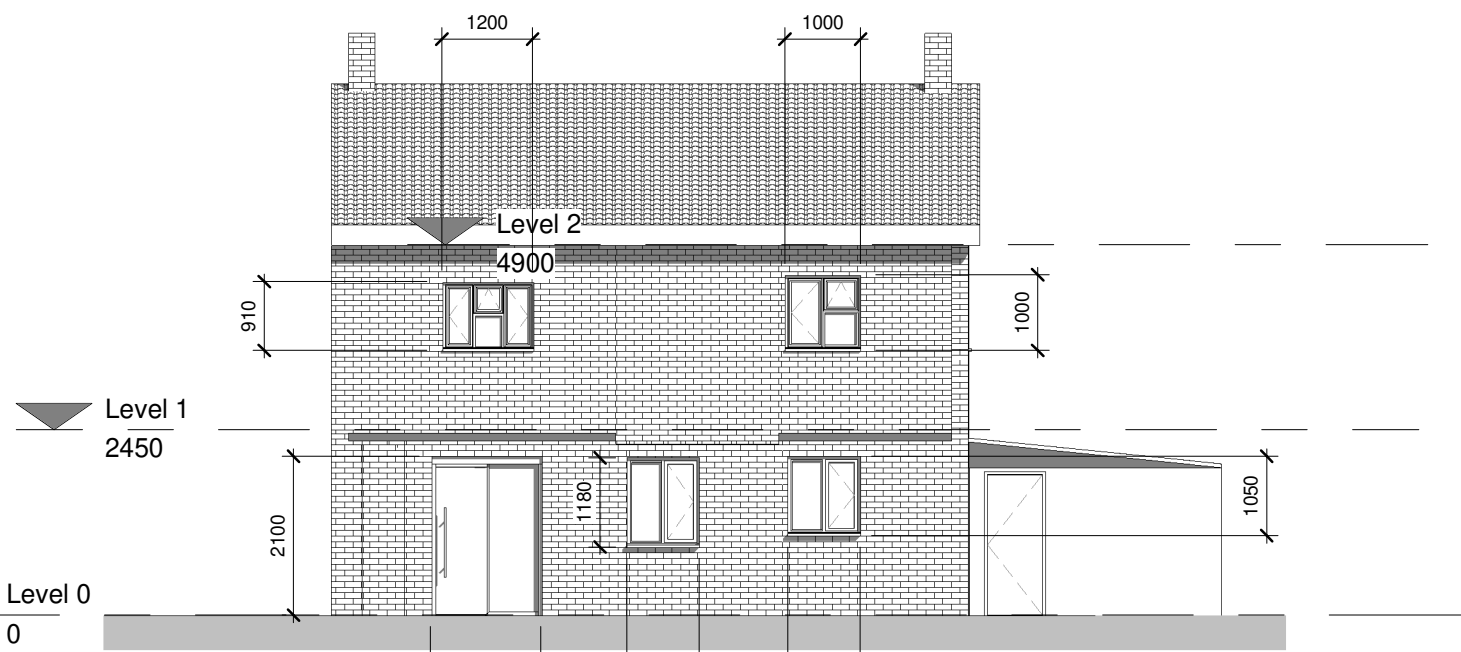
1 Rear elevation - Existing 1 : 100
