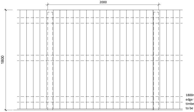
1800mm high feather edge timber fence on timber posts. All timbers to be treated softwood
