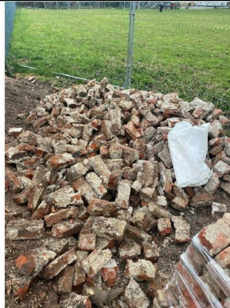
Below ground contaminated bricks
