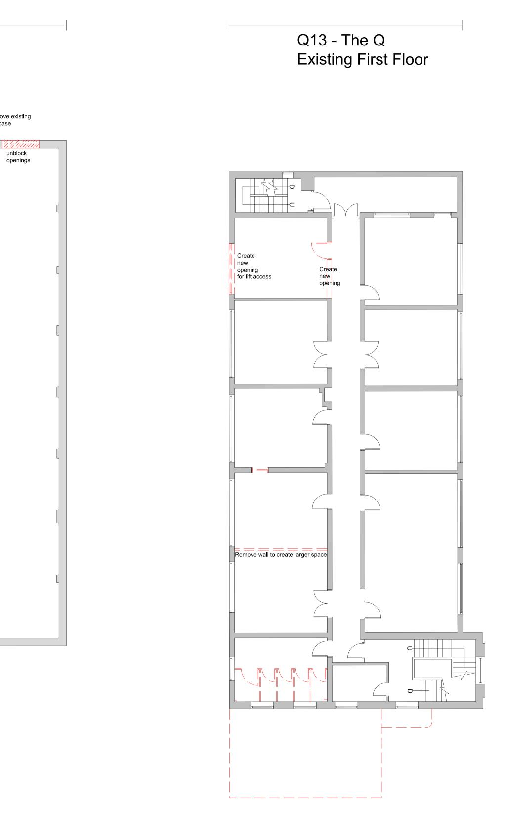
Q14-13 Proposed Primary Demolition\_Void\_FF Scale @ A1 1:100 Job Ref. 00556J Drawing No. 00556J \_ Q14-13\_S08 Revision P1 0 1 2 3 4 5m Scale Bar
