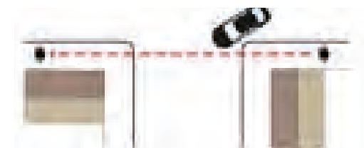
Tighter radii allows pedestrian desire line to be maintained and vehicles turn slowly (10–15 mph)
