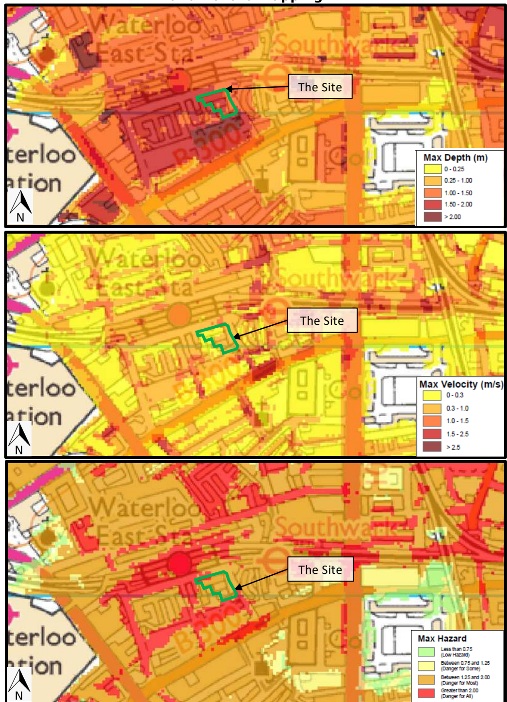
Figure 3-8: Extract of Breach scenario 2100 – Flood Depth, Velocity and Hazard Mapping
