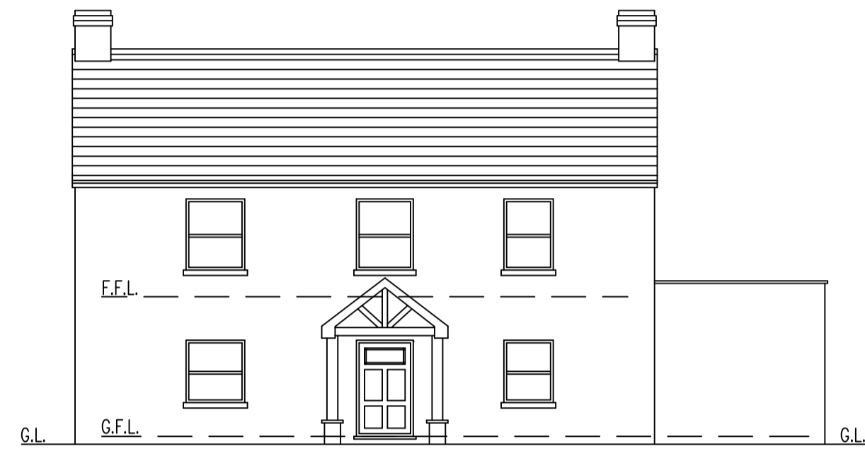
PROPOSED FRONT ELEVATION 1:100
