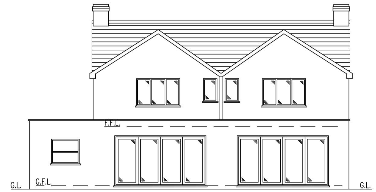
PROPOSED REAR ELEVATION 1:100
