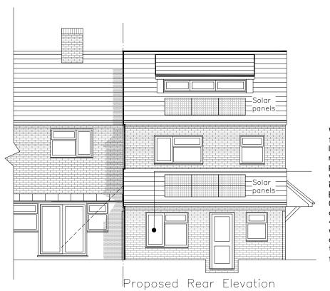
Window to the ground floor bedroom is to be located and sized for means of escape purposes in accordance with the guidance given in paragraph 2.8, Part B1 (e.g. a minimum 0.33 m2 in openable area and at least 450mm high and 450mm wide with bottom of openable area no more than 1100mm above floor level)
