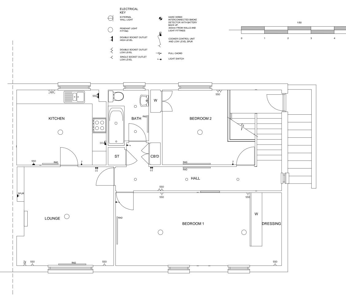
FIRST FLOOR PLAN AS PROPOSED Building (Scotland) Act 2003 note should be made that the relevant person / owner shall be responsible for signing and issuing the completion certificate application to the verifier.
