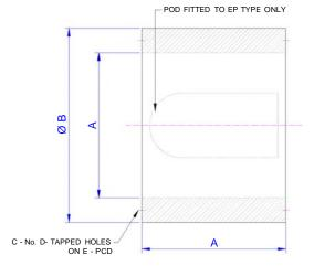
Casing made from galvanized steel, acoustically lined with high density mineral wool covered with cloth to prevent erosion. Acoustic lining retained by perforated steel sheet.
