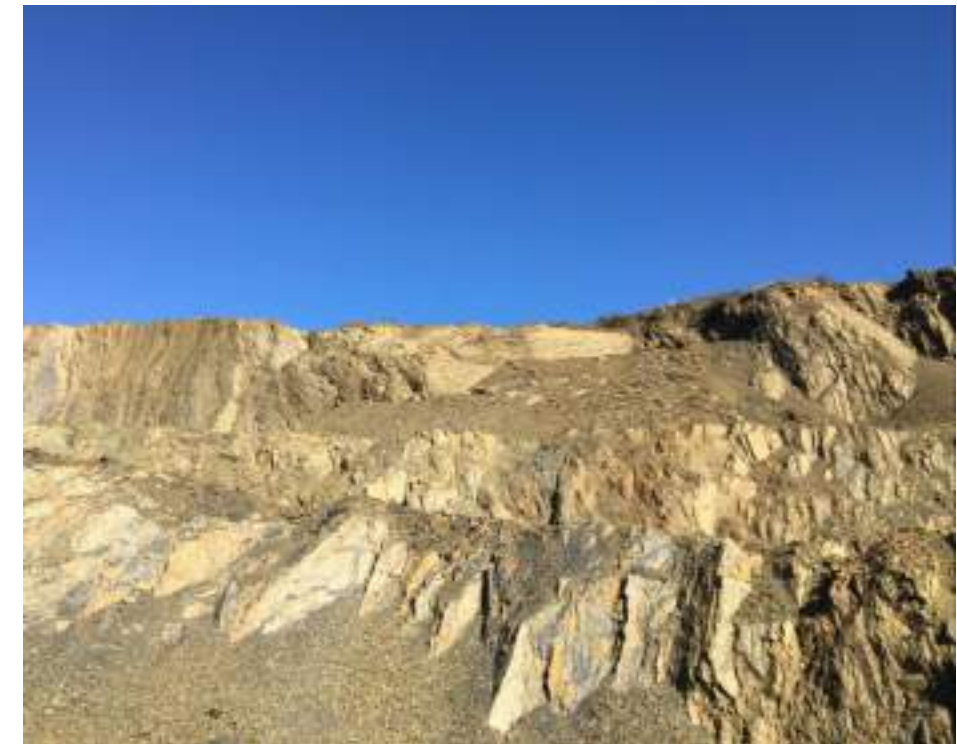
Photograph 4: Faulting and deformation of beds in upper face resulting in planar surface dipping out of the face at approximately 45°.
