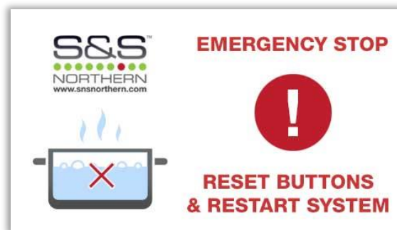
Fig.3.2 Emergency Stop fault display screen.
