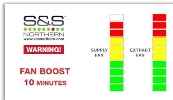
Fig.3.11 Boost activated display screen.
