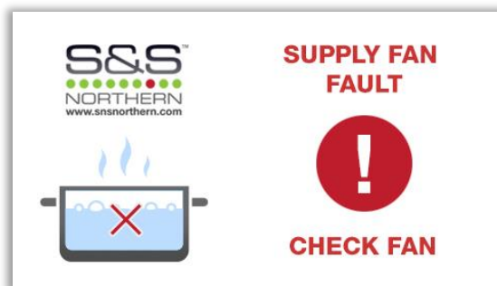
Fig.3.8 Supply fan fault display screen.
