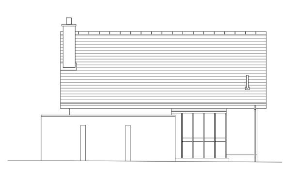
EXISTING SOUTH EAST ELEVATION SCALE 1:100 @ A1
