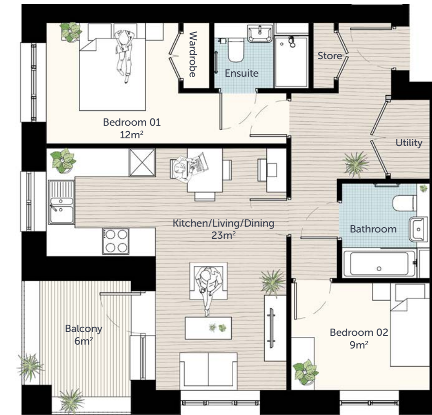
Typical 2B3P Apartment with ensuite 63.5m2
