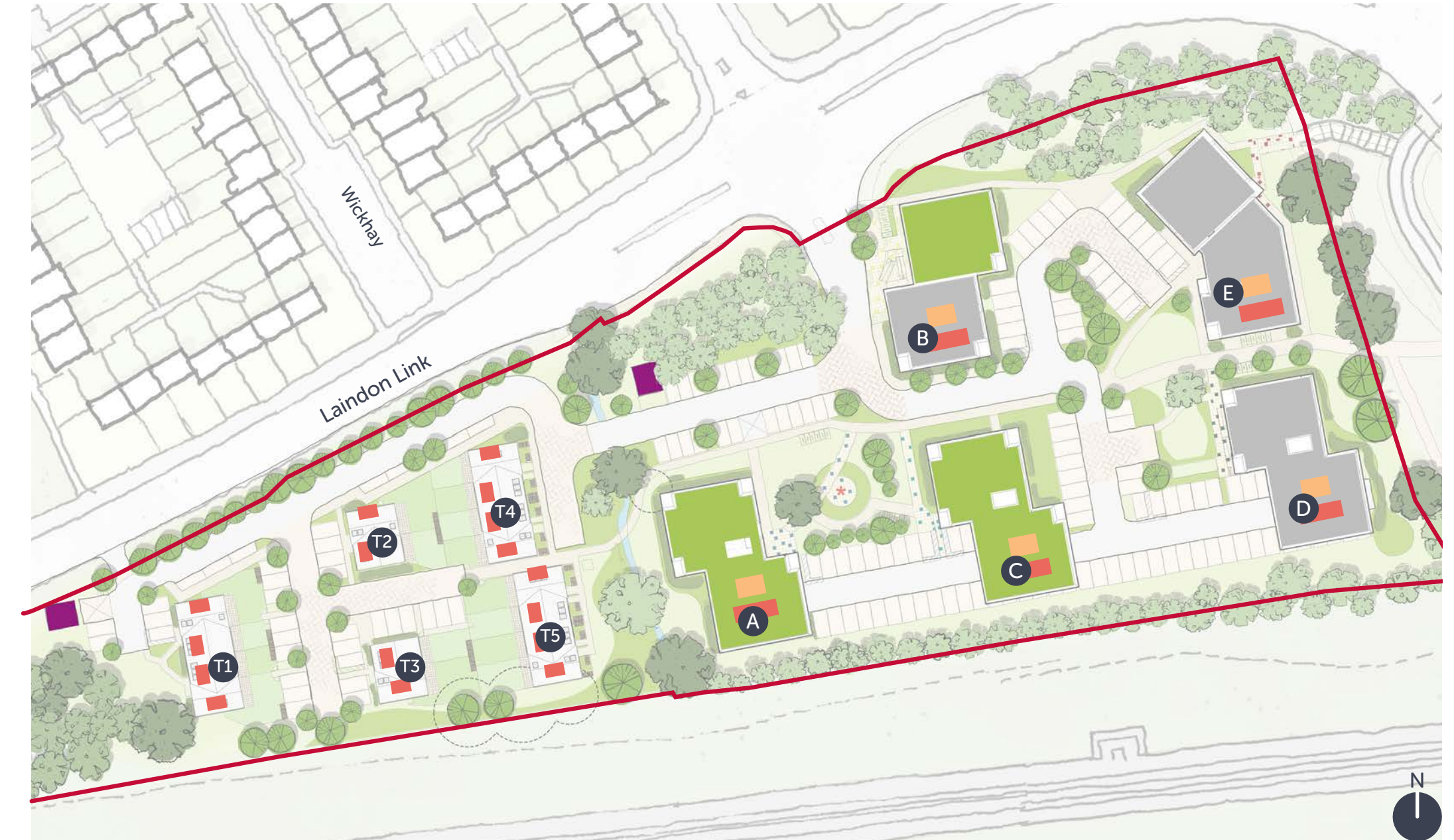
Site Roof Plan with locations of PV and ASHP
