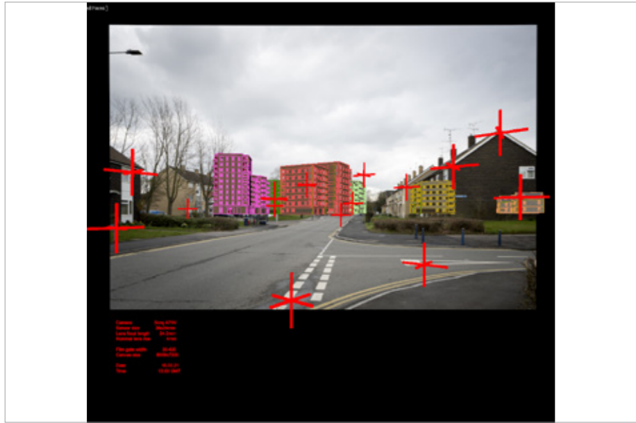
3.7 Screen grab of model matched to photograph
