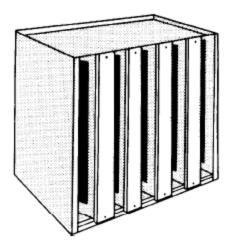
These units are suitable for applications where larger quantities of carbon relative to air flow are unnecessary, or where Modules are unsuitable. They are manufactured from galvanized sheet steel and have slides for the insertion and removal of individual carbon panels. The panels have an aluminum channel frame surround to prevent damage to the panels. when being inserted, and to provide a base for sealing gaskets.
