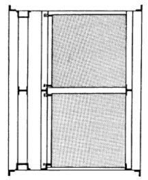
Our standard multiple unit consists of a GSS casing, with 50 x 50 x 6mm RSA flanges both ends. Internally, 50 x 50 x 6mm RSA frames are provided at both ends of the cells, which in turn sit on 10g shelves, welded to both frames. This gives a very rigid internal structure which avoids distortion of the casing.
