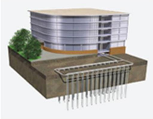
Figure 4: Vertical Closed Loop Ground Source Heating/Cooling System
