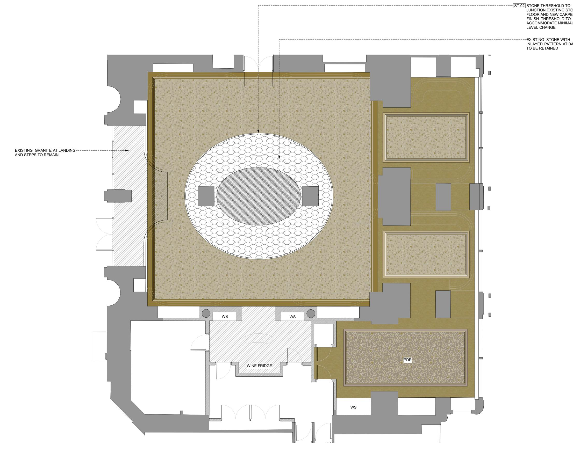
JUNCTION EXISTING STONE FLOOR AND NEW CARPET FINISH. THRESHOLD TO ACCOMMODATE MINIMAL LEVEL CHANGE
