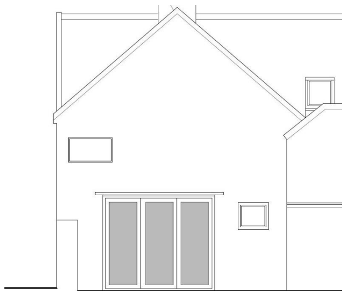
New glazed doors / screen to converted Blacksmiths Forge within existing opening
